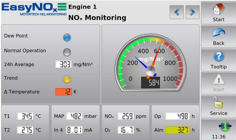
This view displays the current status of the NO<sub>x</sub> monitor. The view varies depending on the set NO<sub>x</sub> monitoring mode. The various parameters of the NO<sub>x</sub> monitor can be set in the *NO<sub>x</sub> Setup* view (see section *Preferences* on page 112). If one of the entries shows the value *A*, the value is outside of the specified range.
